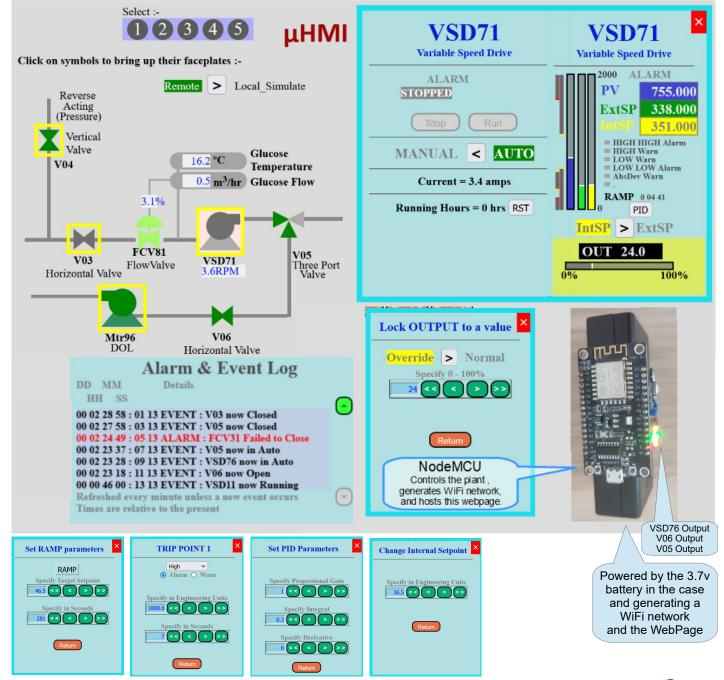
This microHMI shows the capabilities of this technology; accessed from the browser ( on your tablet ) the  $\mu HMI$  ( Human Machine Interface ) connects to the  $\mu PLC$  ( Programmable Logic Controller ) both generated from a NodeMCU board.
